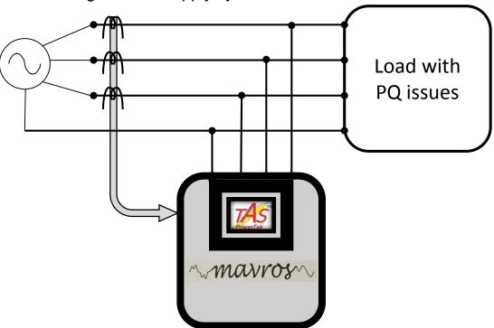
As can be seen from the connection diagram, the said unit is put in parallel with the Electrical Load with Power Quality issues. The said unit can be put in system in either 4-Wire (Ph-1, Ph-2, Ph-3, N) mode which is the most recommended mode or can be put in 3-Wire (Ph-1, Ph-2, Ph-3) mode wherein the Neutral is not connected.
